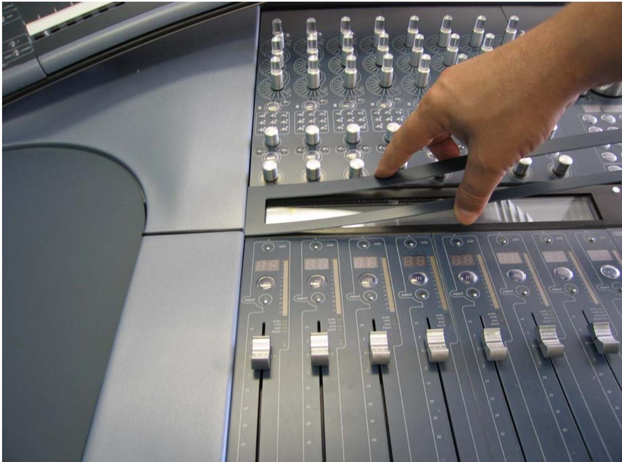
**Plate 8:** The cover strip slides under the cowling of the E96
