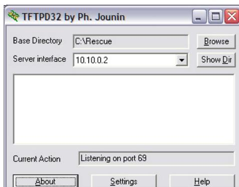
13. Ensure that the Server Interface is 10.10.0.2 -> if the Panel is not connecting correctly to the Ethernet Port you will not see the 10.10.0.2 address appear in the drop down box. If it does not, you will need to check your connection and you MUST close the tftpd32 application and restart it.
